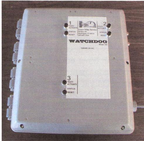
This voice enunciator is designed to allow the operator to record three different 15-second messages for broadcasting over a standard telephone system. These messages can alert personnel of status changes in up to three different monitored pieces of equipment. Another feature permits monitoring of heat detection sensor cable. The belt heat detection and notification of open, short, and fire required by CFR 30 are included.
