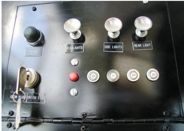
Depress clutch and crank engine until engine starts. *Do not crank engine for more than 20 seconds.* If engine fails to start, Glow Plug the engine and crank engine again. If the engine does not start after several attempts, please refer to Deutz BF4M1011F or the B3.3 Cummins engine Operation Manual.
